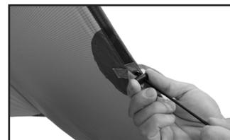
❻ Adjust concealed rubber cord in the seams surrounding the tarp to tension the tarp sides as required.
